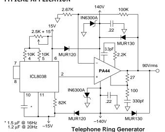
The PA44 is set for a gain of 38.5 boosting the 2.33V signal to 90V. The recommended compensation for gains above 30 is used. If capacitive loading is at least 330pF at all times, the recommended snubber network may be omitted. The 27 ohm resistor sets current limit to a nominal value of 111mA to insure peak currents out of at least 78mA.
